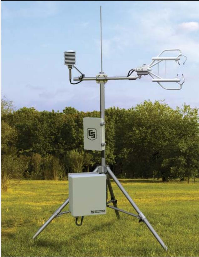
For eddy covariance applications, the CR5000 can measure the EC150 Open-Path CO<sub>2</sub> Analyzer, CSAT3A Sonic Anemometer, and KH20 Krypton Hygrometer then compute fluxes on-line.
